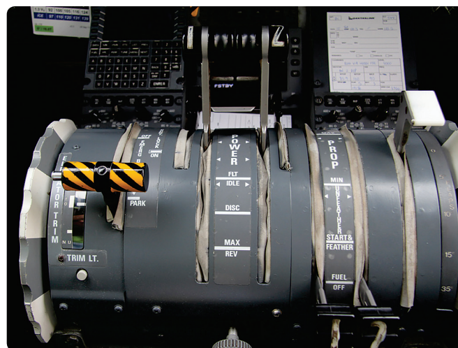
Figure 16-9. A typical dual lever controller on a twin engine Turboprop.
