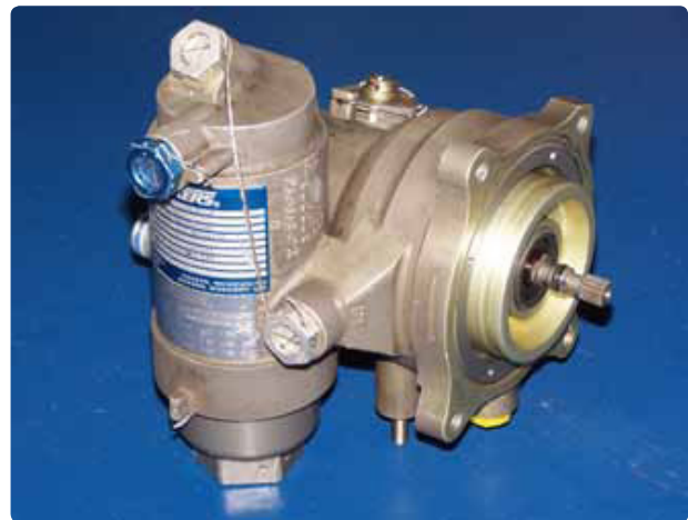
Figure 1-3. Fuel pump and filter.
