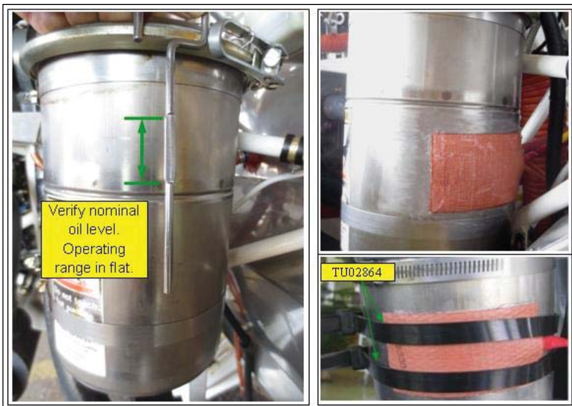
Figure 10 - TEP2688- Pad Heat Element. Install below minimum/nominal operating level. Verify level by holding dipstick outside of tank at the same depth used to the check oil level (flat center portion is operating range, min to max). Note: Correct dipstick has straight top finger loop. Incorrect dipsticks are identified by oval finger loop at top and should be replaced.
