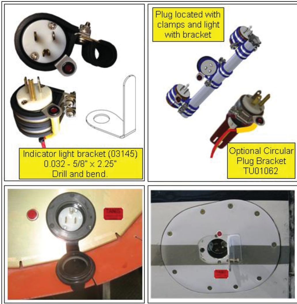
Figure 3 - Examples for locating plug and optional indicator. Top two pictures depict shore plug supplied with kit secured with cushioned clamps and optional circular plug bracket, bottom pictures optional flush plug configurations.
