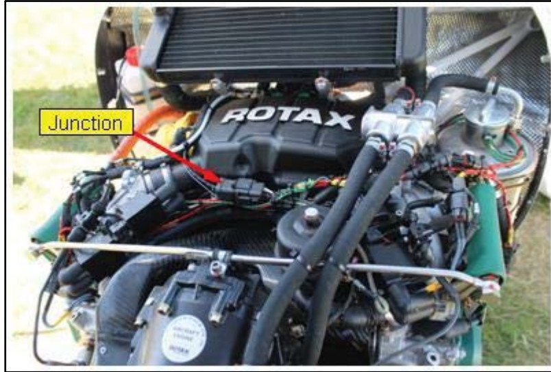
Figure 11 - Routing option: Junction secured with cable ties on existing wiring.
