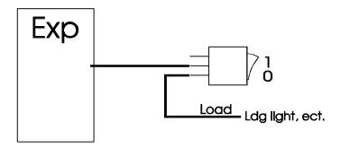
The center terminal of all of the remaining switches connect directly to the switch terminals on the EXP PC Board, (ALT, NAV, STB, AUXFP, LDG1, LDG2, AUX1 and AUX2). The load then connects to the bottom terminal of each switch, as shown above.
