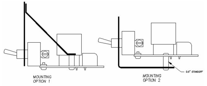
EXP BUS PC BOARD MUST BE MOUNTED AND SUPPORTED TO PROTECT THE ASSEMBLY AGAINST VIBRATION.
