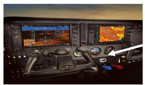
Oximeter and CO detector installed in the middle of the instrument panel
