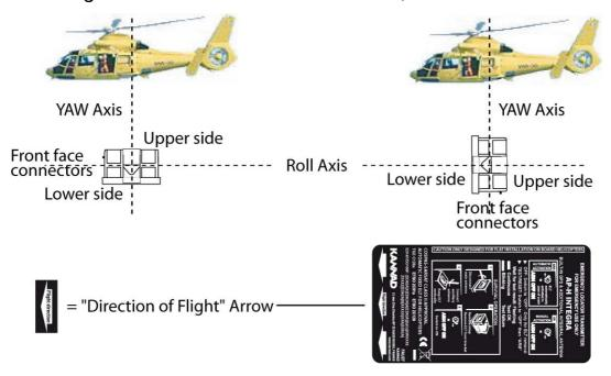
The "Direction of Flight " arrow shall point towards the front or the bottom of the helicopter (and not pointing 45° downwards):
