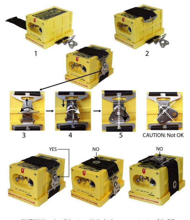
CAUTION: Never install the strap with the latch or grommet on top of the ELT
