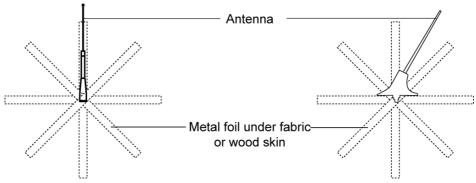
Figure 23: Antenna ground plane for non metallic aircraft
