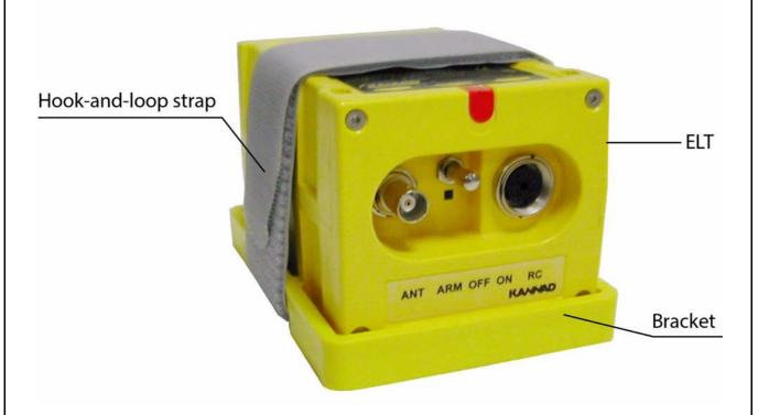
Figure 4: INTEGRA ELT with Mounting Bracket P/N S1840502-02
