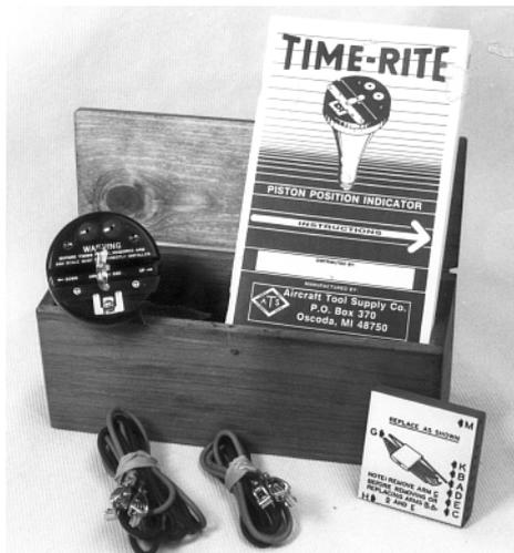
The Model B uses two indicator lights, one shows piston position while the pair is used for synchronizing dual magneto point openings. This is the most versatile model.
