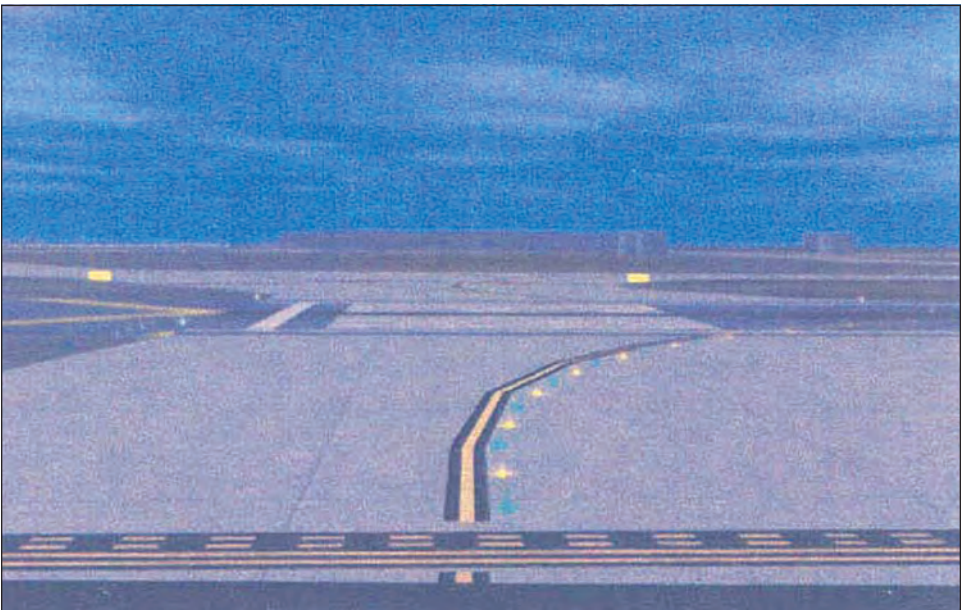
FIGURE 2-1-14 Taxiway Lead-On Light Configuration
