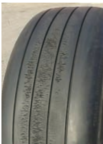
Chevron Cutting not exposing textile can be left in service
