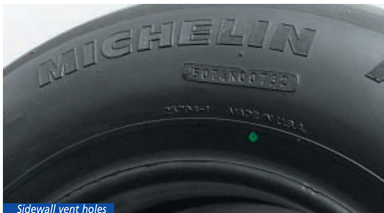
Sidewall vent holes
