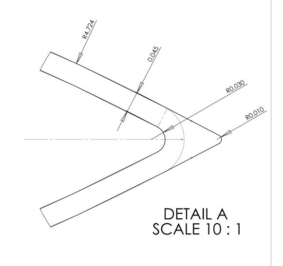
Streamlined Wing Strut Extrusion
