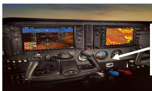
Pulse Oximeter and CO detector installed in the middle of the instrument panel
