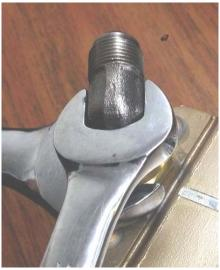
Oil Coolers with hex nut style inlet/outlets must always be installed by **holding the nut with a wrench while threading the fitting in with another wrench.** This is critical to prevent the flexible aluminum oil cooler from bending and possibly weakening or splitting apart the end sections. Thread sealant must be used on fittings.
