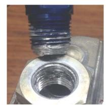
Even when thread sealant is applied, aluminum fittings often "pick up" and destroy the threads. Because of this,
