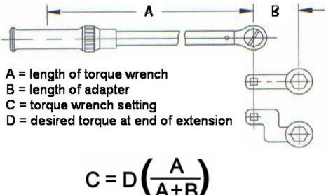
NOTE: Regular socket extensions which extend directly under the drive head along the axis of rotation of the ratchet do not affect the calibration of the torque wrench.
