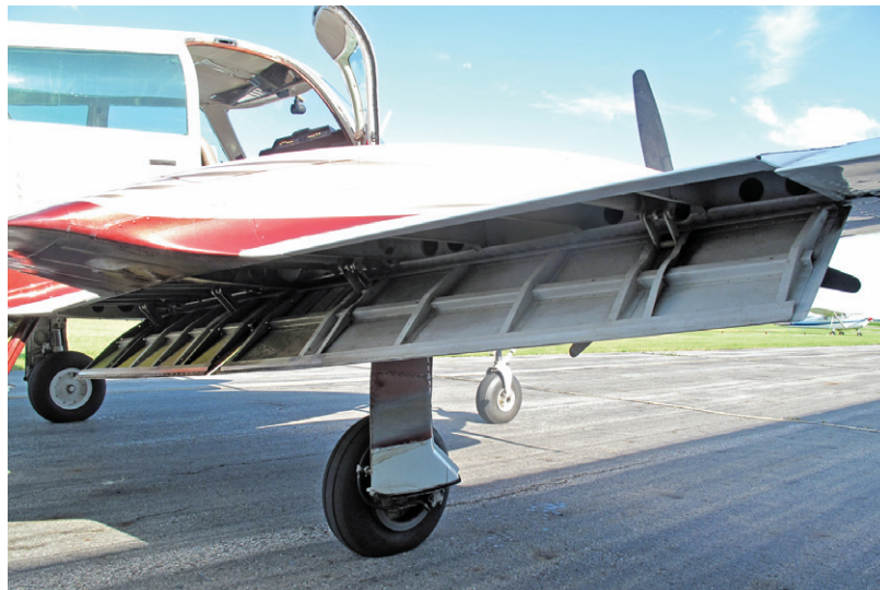
Figure 1-6. Cessna split flap system.
