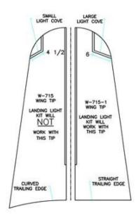
**RV-7/8**: Any RV-7/8 that was built with the W-715-1 wingtip fairings can accept the Aerosun Vx. If your airplane has the older W-715 fairings then an upgrade to the W-715-1 wingtip fairings to be able to install the Aerosun Vx. All kits that were shipped from 2005 on should have the W-715-1 fairings.
