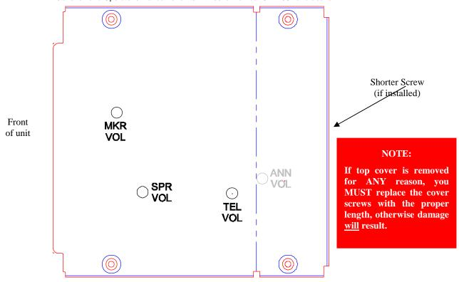
Figure 2-4- PMA8000BT Adjustments, top cover
