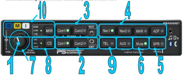
Figure 3-1 PMA8000BT Operating Controls
