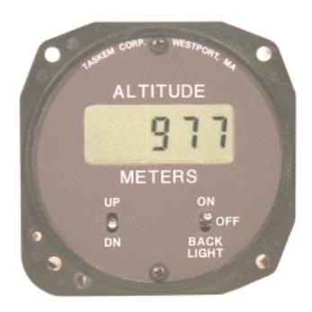
The altitude range extends from below sea level to well above the need for supplementary oxygen. The limits are -1,000 to +19,990 feet or -305 to +6,093 meters. Altitude increments are in 10 feet or 1 meter steps. This fine resolution, particularly in meters, provides a useful tool for land surveying.
